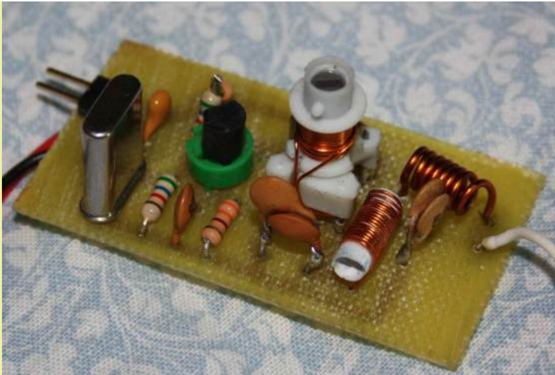
Here is the circuit made by Lucian Papadopol iz6nnh@gmail.com He has created capacitor values by paralleling two values.
